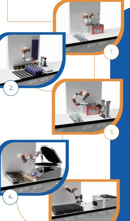
**1. Ultrasonic bath sample exchanger:** Revolutionizes sample preparation by providing an automated, efficient, and precise method for cleaning and exchanging samples within an ultrasonic bath, reducing manual handling and improving throughput.
