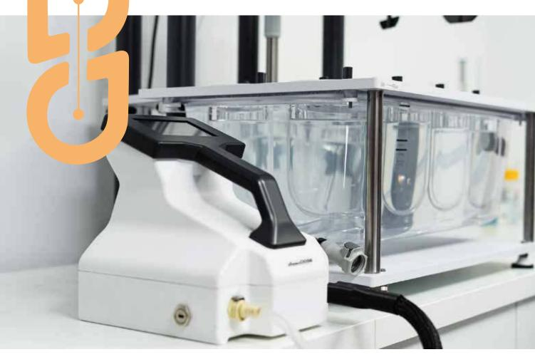
Volumetric medium dispensing with accuracy better than 0.5% for 900ml Battery-powered, handy portable unit Intuitive user interface Three different dispensing speeds Appropriate for foaming medium Easy dispensing history review Easy cleaning procedure
